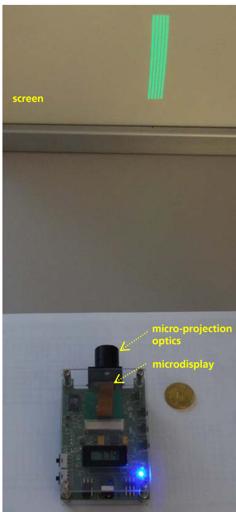
Figure 1: HYPOLLED microdisplay test chip and pattern operating with micro-projection optics
